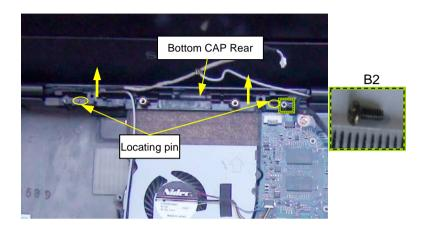
Remove one screw. Remove Bottom CAP Rear. Note two Locating pins.
