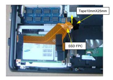
Peel off one Tape. Disconnect the SSD FPC vertically.
