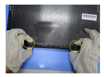
Release the clips from two side carefully.
