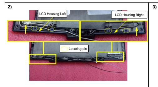
Lift up LCD Housing Left and LCD Housing Right. Note the Locating pins.
