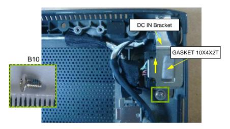
Remove one screw and lift up DC IN Bracket. Remove the gasket.
