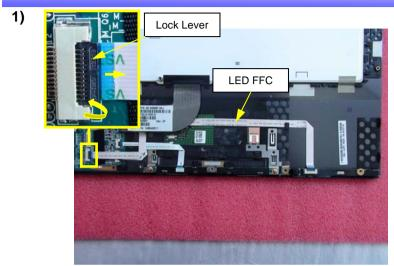
Raise the Lock Lever as the arrow and disconnect LED FFC from MS/SD Daughter Board.
