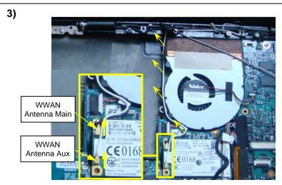
Pull out the WWAN Antenna from WWAN Card vertically.
