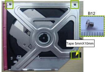
Remove the Tape. Remove three screws.
