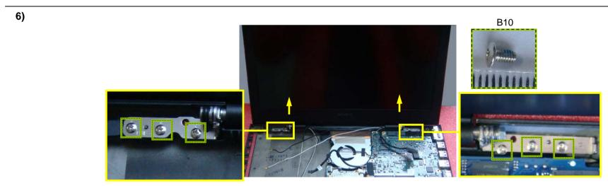
Holding the LCD Unit, remove six screws.
