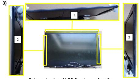
Release the clips of LCD Bezel gently from the outside edges as picture shown.
