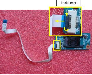
Raise the Lock Lever as the arrow and disconnect SIM FFC from SIM Card.
