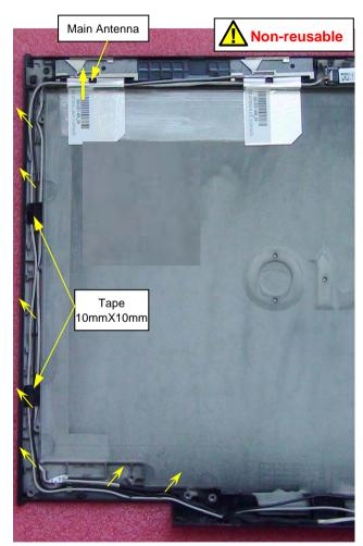
Peel off two Tape. Peel off the Main Antenna from display housing and then remove the Main Antenna. Note the Antenna's route.
