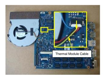
Disconnect Thermal Module Cable horizontally from Main Board.
