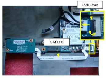
Raise the Lock Lever as the arrow and disconnect SIM FFC from Docking Daughter Board.
