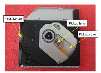
Don't touch the Pickup lens. Be careful handling of below point: ODD Flame, pickup Cover, ODD Mount and ODD FFC.
