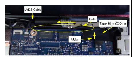
Peel off the Tape. Lift up LVDS Cable vertically with Mylar. Pull out the LVDS Cable from the Hole.
