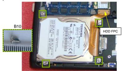
Disconnect the HDD FPC from Main board vertically. Remove four screws.
