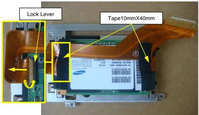
Peel off two Tapes. Raise the lock lever as the arrow. Disconnect one side of SSD FPC from one SSD horizontally.
