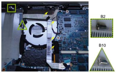
Remove two screws of different kinds. Lift up ODD FFC Holder. Note ODD FFC is fixed thermal Module by double tape.
