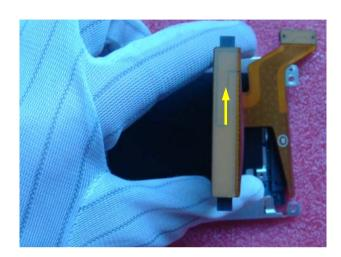
While one hand holding the SSD, the other hand disconnect SSD FPC from the SSD.
