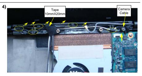
Peel off one Tape. Disconnect Camera Cable horizontally. Remove the cables from Rear cap. Note the cables' route.
