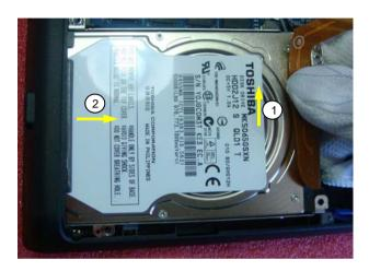
Lift up HDD in the direction of arrow 1 and then pull out it in the direction of arrow 2.
