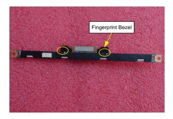
Release two clips and then remove the Fingerprint Bezel. Note the Fingerprint Bezel fixed Fingerprint Daughter Board with TAPE 5X3.
