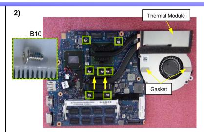
Turn the unit over. Remove seven screws and lift up Thermal Module.
