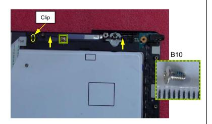
Remove one screw and remove the Speed Daughter Board.
