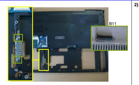
Turn the Bottom over. Remove two screws.
