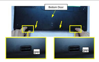
Holding the two gaps, push out Bottom Door horizontally to remove.
