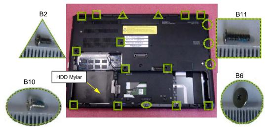
Remove eighteen screws of four kinds. Remove the HDD Mylar.
