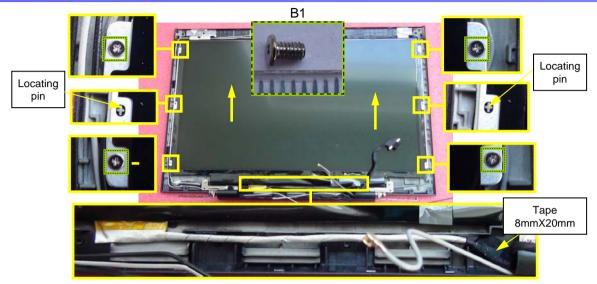
Remove four screws. Peel off one tape. Take up the LCD Panel with two hands. Note the LVDS Cable's route and the Locating pins.
