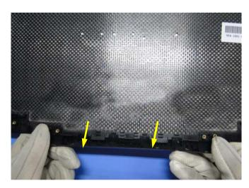
Remove Hinge Cover from display housing as picture show.
