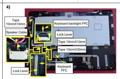
Peel off four Tapes. Disconnect Speaker Cable, Keyboard backlight FPC and Keyboard FFC.
