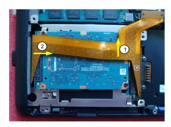
Lift up SSD in the direction of arrow 1 and then pull out in the direction of arrow 2.
