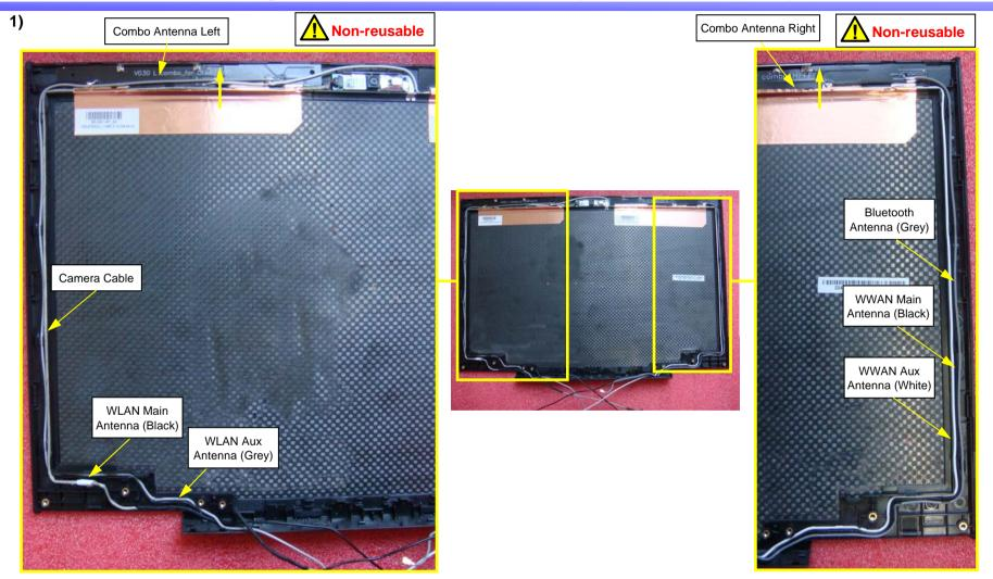
Peel off Combo Antenna Right and Combo Antenna Left. Note the antennas' route.
