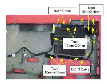
Peel off seven Tapes. Remove DC IN Cable and RJ45 Cable.
