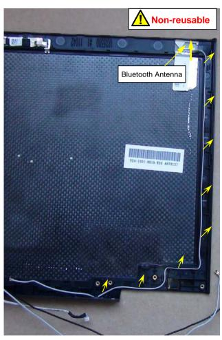
Peel off the Bluetooth Antenna from display housing and then remove the Bluetooth Antenna. Note the Antenna's route.
