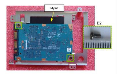
Turn the unit over. Remove two screws and remove the SSD.
