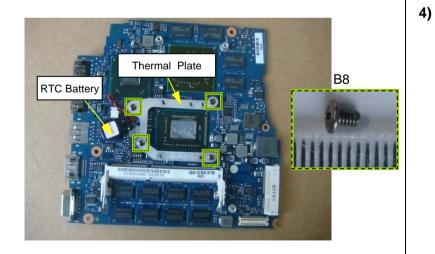
Remove four screws and then remove Thermal Plate.
