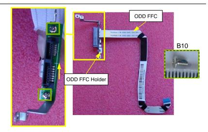
Remove two screws. Lift up ODD FFC.
