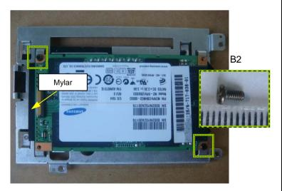
Turn the SSD over. Remove two screws and then remove the other SSD.
