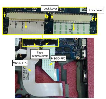
Peel off two tapes. Unlock the Lock Lever, then disconnect MS/SD FFC MS/SD FPC from Main Board horizontally.
