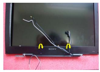
Release the clips of LCD Bezel bottom side gently from the inside edges.
