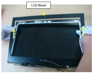
Remove LCD Bezel carefully with two hands.
