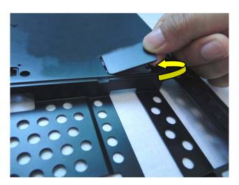
Turn over Bottom, remove SIM Card Door as picture shown. 36
