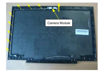
Remove the Camera Module. Note the Camera Cable's route.
