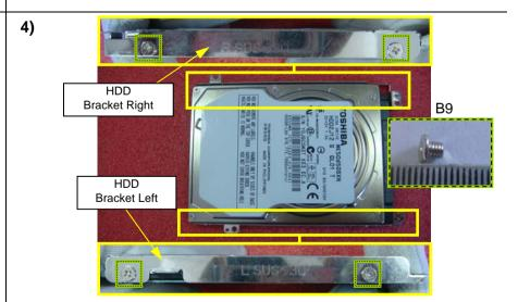
Remove four screws and lift up HDD Bracket Right and Left.
