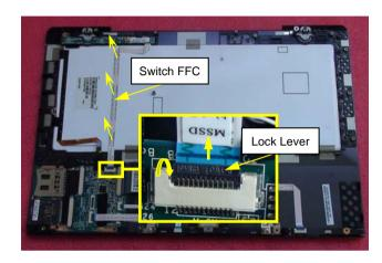
Raise the Lock Lever as the arrow. Disconnect Switch FFC from MS/SD Daughter Board. Note Switch FFC is fixed to Palmrest with double tape.
