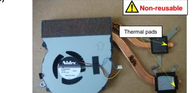
The Thermal pads are attached on the bottom of the Thermal Module. 40
