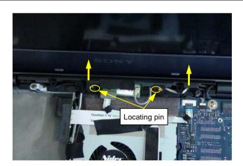
Lift up Hinge Top Cap. Note two Locating pins.
