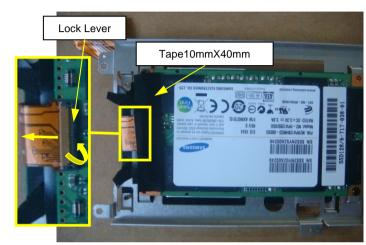
Turn the SSD over . Peel off one Tape.
