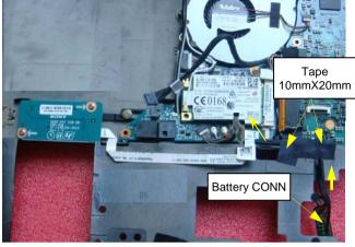
Turn the unit over. Peel off two Tapes. Pull out the Battery CONN.
