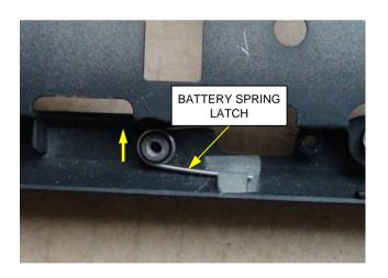
Remove BATTERY SPRING LATCH.
