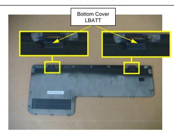
Remove the Bottom Cover LBATT. Note the Cover LBATT fixed Bottom Door with adhesive tapes .
