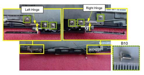
Remove six screws. Lift up Right Hinge and Left Hinge.
