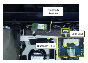
Raise the lock lever as the arrow, disconnect Bluetooth FFC from Main Board. Pull out the Bluetooth Antenna vertically.
