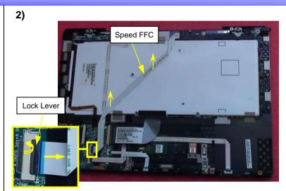
Raise the Lock Lever as the arrow and disconnect Speed FFC from MS/SD Daughter Board. Note Speed FFC is fixed to Palmrest with double tape.
