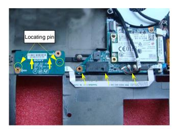
Remove the SIM Card. Note Audio Board FFC is fixed to Bottom with double tape.
