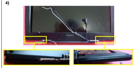
Release the clips of LCD Bezel blow side gently from the outside edges as picture shown.
