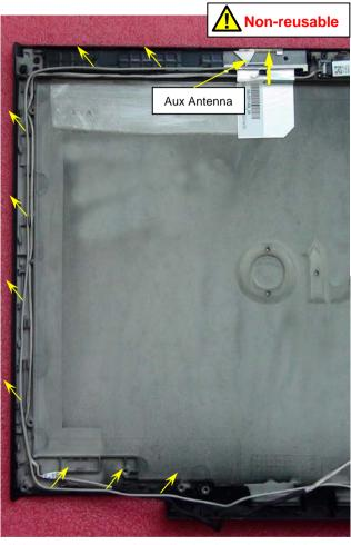
Peel off the Aux Antenna from display housing and then remove the Aux Antenna. Note the Antenna's route.
