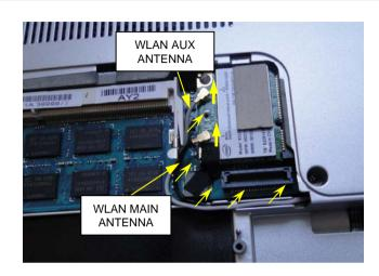
Pull out WLAN ANTENNA vertically from WLAN CARD.
