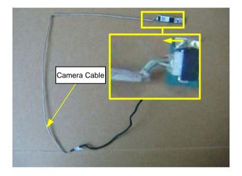
Disconnect Camera Cable from Camera Module horizontally.
