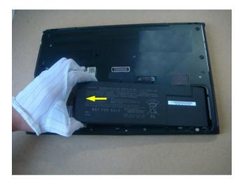
Pull out the Battery pack in the direction of the arrow.
