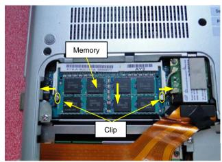
Gently press the clips away from the Memory Module and lift the Memory Module from the system.
