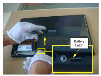
While one finger pressing the Battery Latch, the other hand lift the Battery Pack up.
