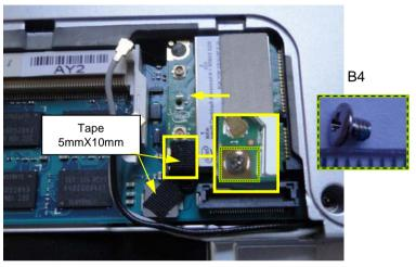
Peel off the TAPE. Remove one screw and then remove the WLAN CARD in the direction of arrow.
