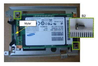
Remove two screws and then remove the SSD.
