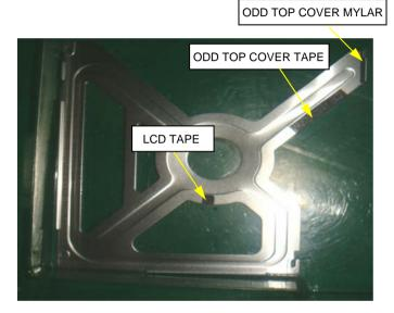
Note the position of LCD TAPE, ODD TOP COVER TAPE, ODD TOP COVER MYLAR.
