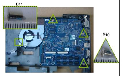
Remove four screws. Note there are two different kinds of screws.
