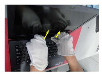
Turn the Unit over. Open the LCD section.
